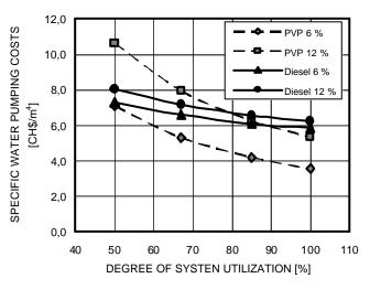
compared with the smallest available diesel pump as a function of the degree of system utilisation for different interest rates.
