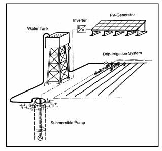
PVP tank irrigation systems operate at constant pressure of approximately 0.2 - 0.5 bar depending on the height of the water tank and with a rather constant water flow. Irrigation is regulated by hand valves
