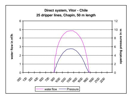
Drip irrigation saves a considerable amount of water compared to other irrigation techniques. Furthermore, it has a rather low operating pressure. Both features reduce the energy demand and make drip irrigation particularly suitable for photovoltaic pumping systems.
