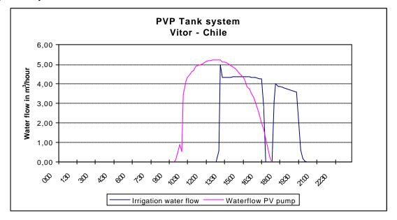
In the second case, the PVP injects the water directly into the irrigation system. As pertinent experience in Chile shows, this can reduce the initial capital outlay by as much as 35%. However, due to daily fluctuations of global radiation, these systems operate at variable system pressures and water flows.
